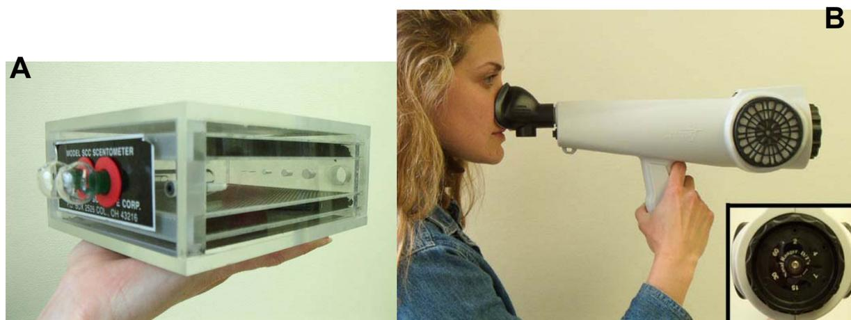
Figure 3. (A) The Scentometer Field Olfactometer (Barnebey Sutcliffe Corp.). Note the two glass nostril ports to the left and the series of orifices at the back of the unit to the right of the photo. (B) The Nasal Ranger Field Olfactometer (St. Croix Sensory). The inset picture shows the orifice dial, which is located at the right side of the Nasal Ranger in this photo.
